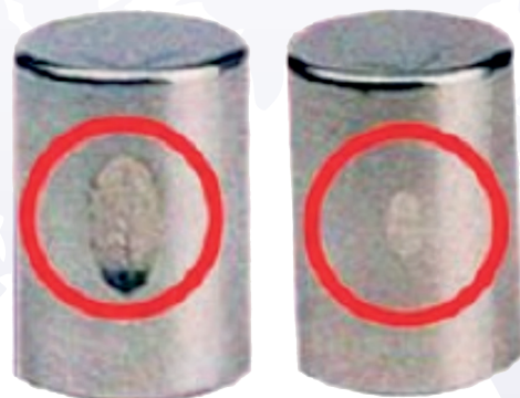
In comparison: abrasion without (left) and with micfil ultra fine filter after 4000 h without oil change (right).
